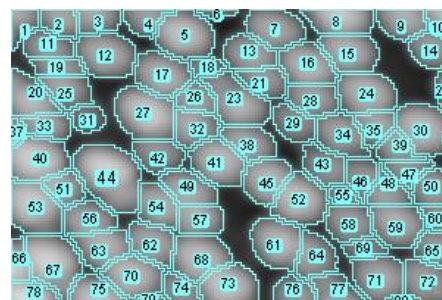
Segmented Particles (ROIs obtained with Analyze▷Analyze Particles...)
