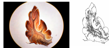
Original image and binary outline created in ImageJ using thresholding, dilation, and outlining.
